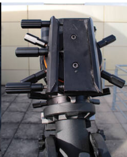
Fig. 14: CGE PRO clamp on the mounting
