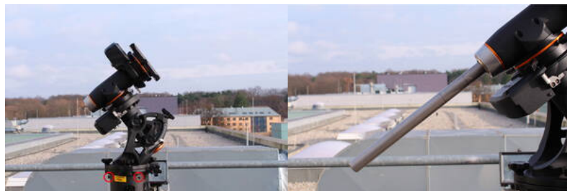
Fig. 5: CGE PRO mounting on electronic box and tripod (the red circles indicate the three bolts to be fastened)
