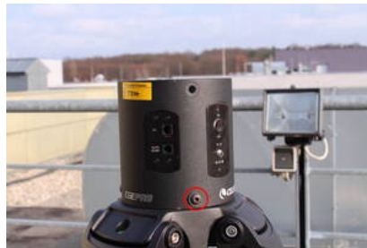
Fig. 2: tripod with electronic box (the red circles indicate the three bolts to be fastened)
