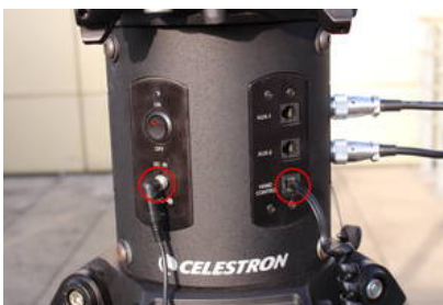
Fig. 12: ports for power supply (left) and terminal (right) at the electronic box
