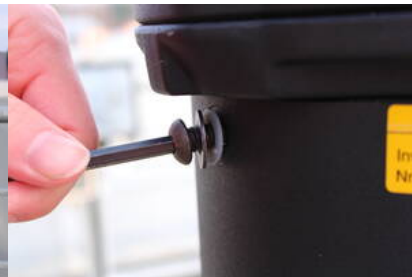
Fig. 3: One of the electronic box bolts
