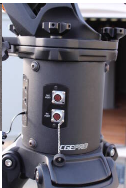
Fig. 8: electronic box with ports for the cable to the engines
