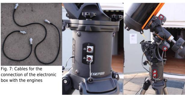
Fig. 8: Electronic box with ports for the cables
