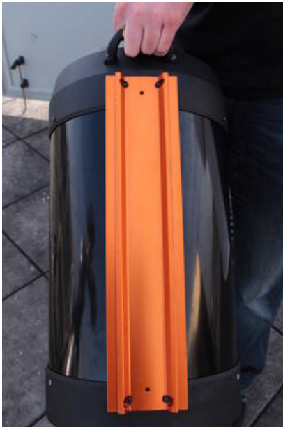
Fig. 13: Dove tail on the tube
