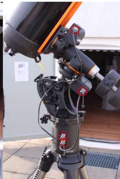
Fig. 9: CGE PRO with the cable attached
