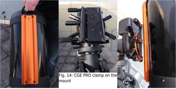
Fig. 13: Dove tail on the tube
