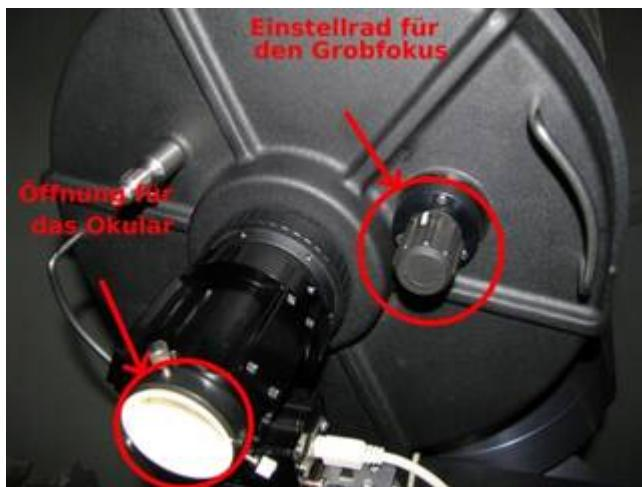
Coarse focus (The white dust protection has been replaced by a small black box which contains a desiccant to keep the telescope dry).
