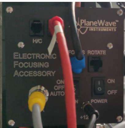
Fig. 2: The control box of the EFA
