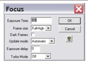
The settings should be similar to the example shown on the image above. In this operation mode, the camera will repeatedly take images of a certain Exposure Time (0.5s in the example above). The individual exposures will be automatically downloaded and displayed. Now the telescope can be focused using *CW3* or the hand terminal for the EFA.
