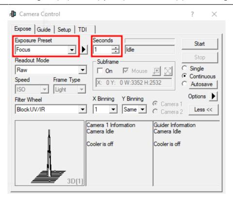
After a click on Start images are continuously taken and displayed. Now the telescope can be focused by means of *CW3* or the hand terminal of the EFA. To find the coarse focus, it is recommended to first approach a bright star and to focus in such a way that the diffraction ring disappears. Rough values for the focus with the different instruments and eyepieces can be found in the table above.
