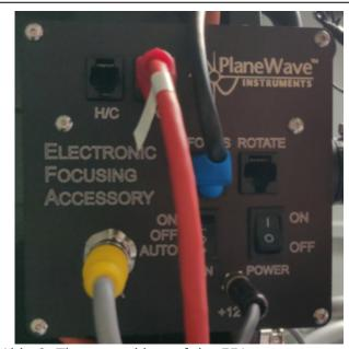
Abb. 2: The control box of the EFA
