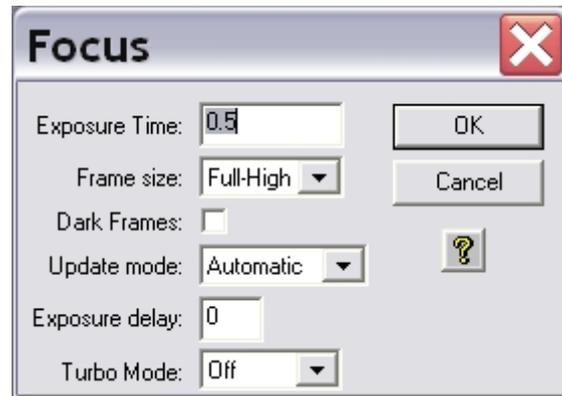
The settings should be similar to the example shown on the image above. In this operation mode, the camera will repeatedly take images of a certain Exposure Time (0.5s in the example above). The individual exposures will be automatically downloaded and displayed. Now the telescope can be focused using CW3 or the hand terminal for the EFA.
