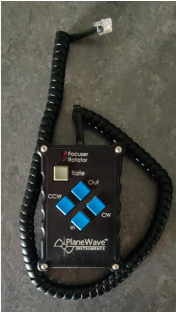
Fig. 1: Hand terminal for the EFA
