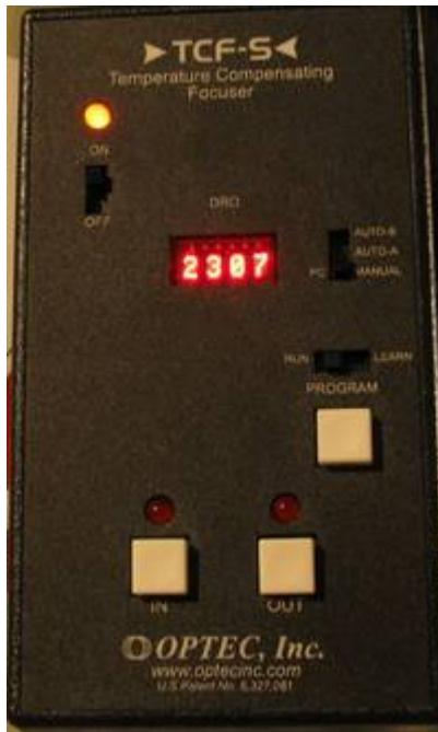
Control unit for the motorized focus (ideal for precise adjustments)
