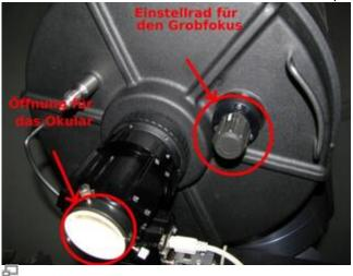
Manual focus knob (for the rough adjustments; the white dust cover has been replaced by a black nozzle that contains desiccant, which keeps the telescope dry)
