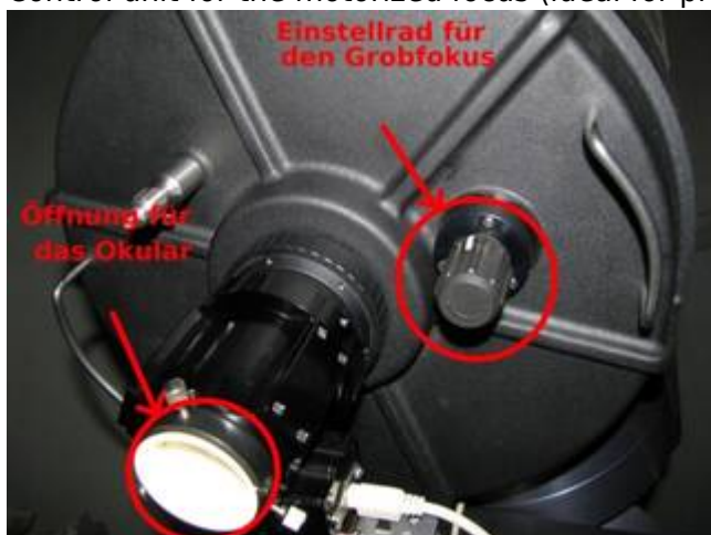
Manual focus knob (for the rough adjustments; the white dust cover has been replaced by a black nozzle that contains desiccant, which keeps the telescope dry)
