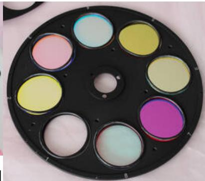
3. Filter holder with filters and spacer rings
