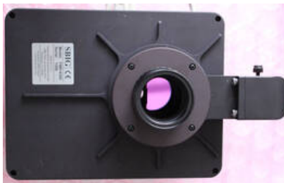
7. Filter wheel with the OAG and T2 adapter
