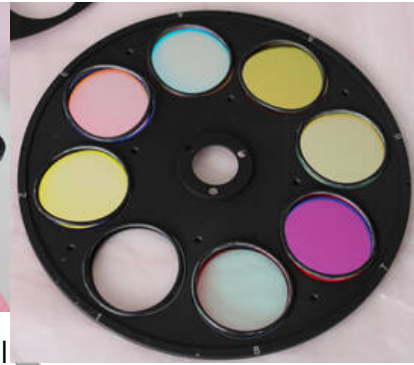
3. Filter holder with filters and spacer rings
