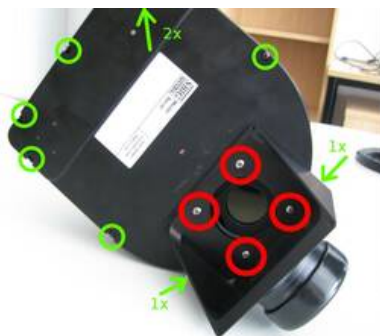
3: Screw positions on the filter-wheel backplate (green circles) and the AO case (red circles)
