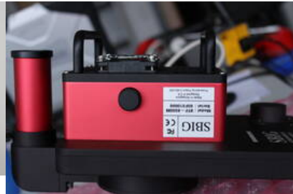
9. STF-8300 with filter wheel, OAG, and ST-i
