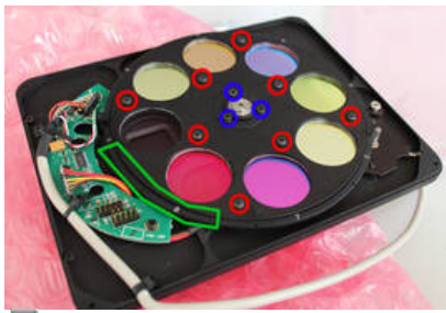
4. Filter wheel with inserted filter holder (the red circles mark the screws that attach the cover to the filter holder, the blue circles mark the screws that attach the filter holder to the backplate of the filter wheel)
