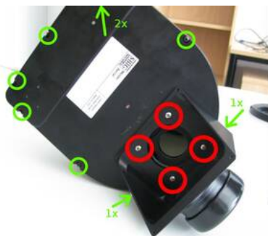
3: Screw positions on the filter-wheel backplate (green circles) and the AO case (red circles)
