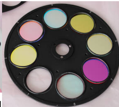
3. Filter holder with filters and spacer rings
