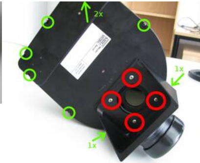
3: Screw positions on the filter-wheel backplate (green circles) and the AO case (red circles)
