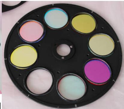
3. Filter holder with filters and spacer rings
