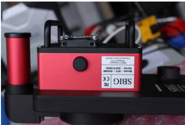
9. STF-8300 with filter wheel, OAG and ST-i
