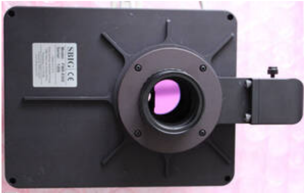
7. Filter wheel with OAG and T2 adapter
