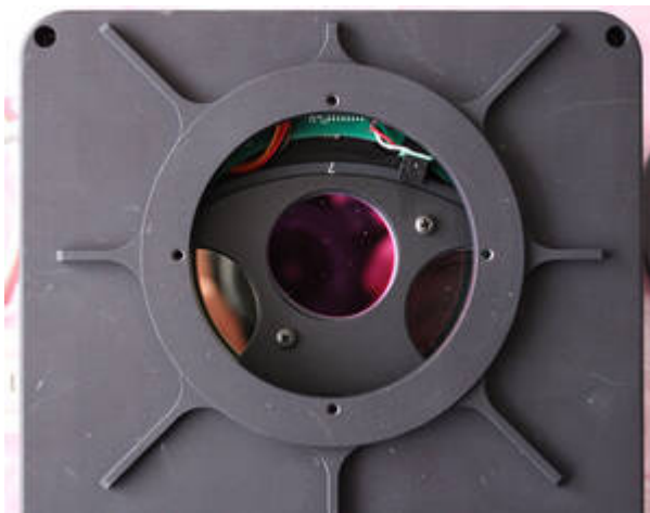
5. Filter wheel with cover
