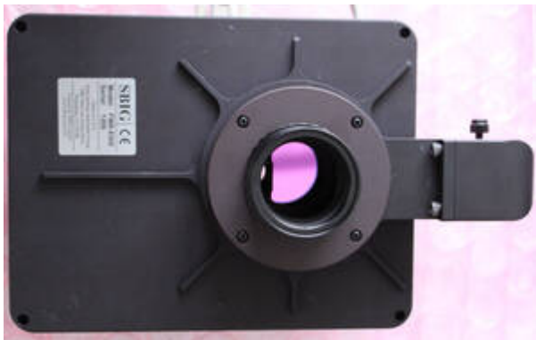
7. Filter wheel with OAG and T2 adapter
