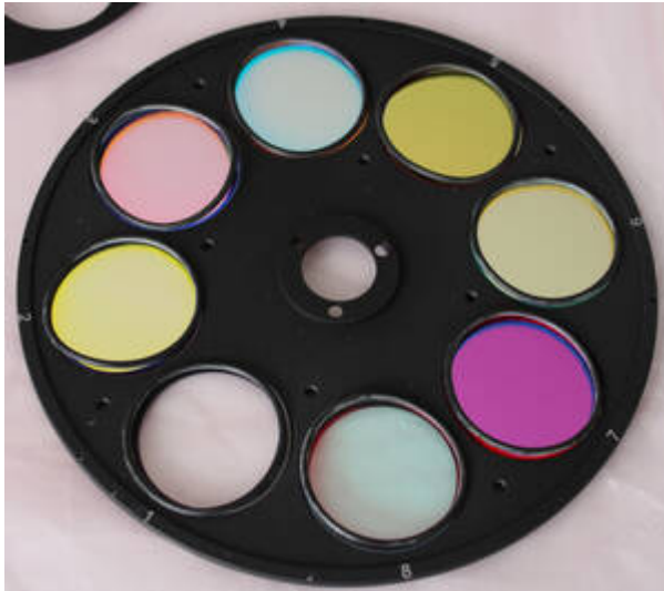
3. Filter holder with filters and spacer rings
