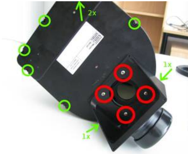
3: Mount the filter wheel
