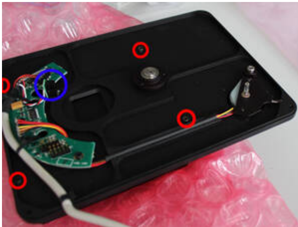
2. Backplate of the filter wheel mounted to the SFT-8300 (the red circles mark the corresponding screws, the blue circle mark the sensor for the filter wheel position)
