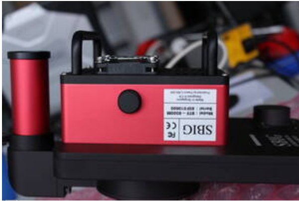
9. STF-8300 with filter wheel, OAG and ST-i
