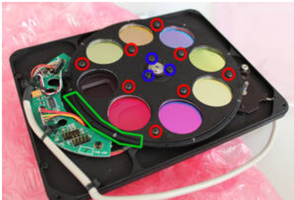
4. Filter wheel with inserted filter holder (the red circles mark the screws that attach the cover to the filter holder, the blue circles mark the screws that attach the filter holder to the backplate of the filter wheel)
