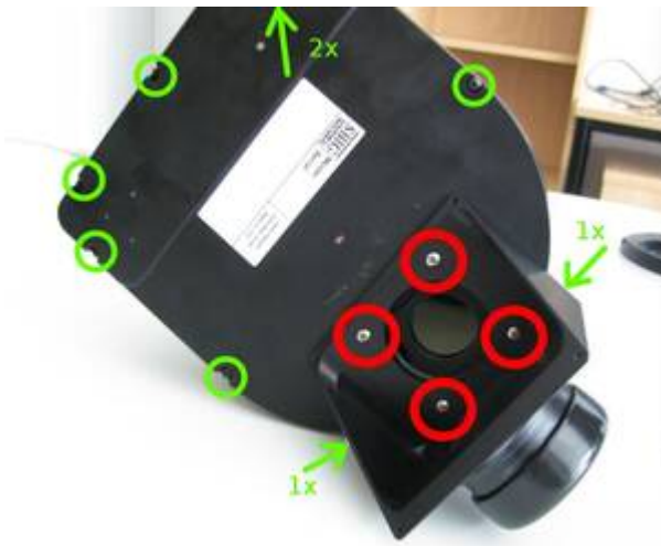
3: Mount the filter wheel
