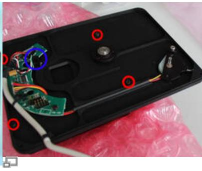
2. Backplate of the filter wheel mounted to the SFT-8300 (the red circles mark the corresponding screws, the blue circle marks the sensor for the filter wheel position)
