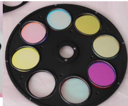
3. Filter holder with filters and spacer rings
