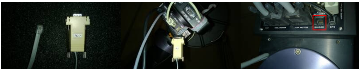
1: Guider cable with the RC-7 plug 2: A07 CFW8 SCOPE Port of the camera with attached Guider cable 3: GUIDER Port of the mount
