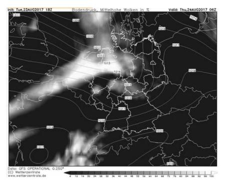
In the upper left corner you can find the time when the calculation was performed (Init), while the time for which the forecast is valid (Valid) can be found in the upper right corner. In between you can find the requested quantity (in German). Below the map a scale is plotted, that helps interpreting what is shown on the map.
