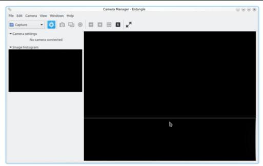
To establish a connection, the item *Connect* can be found in the *Camera* menu. A small window will now show a list of all available cameras. With a click on Connect the program should establish the connection.
