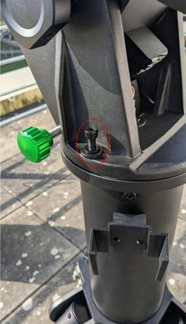
A close-up photograph of the telescope mount. A red circle highlights a hex screw being inserted into a hole on the side of the mount. A green adjustment knob is visible on the left side of the frame. |
