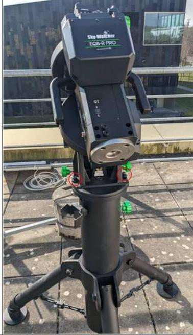
A photograph showing a black telescope mounted on a tripod. The telescope is in its folded position. The mounting bracket is attached to the tripod head. The telescope body has 'Sky-Watcher EQ8-R PRO' printed on it. The setup is on a concrete surface. |
